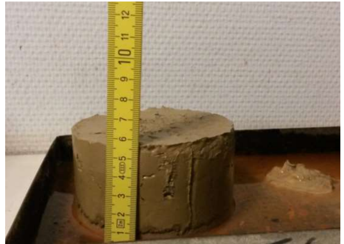
Self Sealing after water access. Constrained volume change
